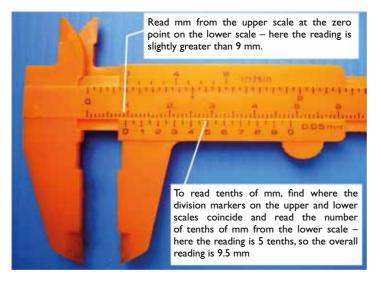
illustrated here reads 9.5 mm. Because RCD is a small value, it must be measured with high accuracy. For best results, measure RCD twice by turning the callipers at right angles and then use the average reading.
