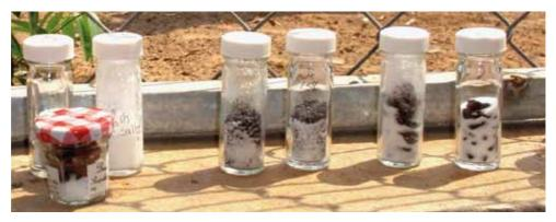
Salt can also be used in a crude test for moisture content. Quarter fill a small glass jar with very dry table salt, add about an equal volume of seeds and shake. If the salt forms clumps, the eRH is higher than 70%. If the salt remains free flowing, then the seeds can be stored, at least in the short term.
