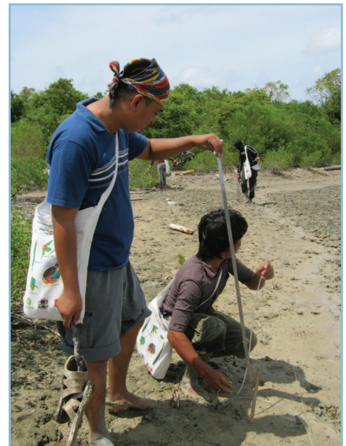
Fig. 5.14 Using a water level to measure substrate elevations towards the landward edge of the mangrove which is rarely inundated by high tide.
