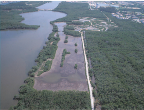
Fig 8.15 The intentional design of open water refugia in a mangrove rehabilitation project, increases fisheries habitat and can speed up the achievement of a functional fisheries equivalent, and wading seabird feeding habitat, common objectives of mangrove restoration projects.
