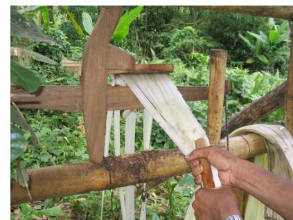
Hand stripping using serrated blade
