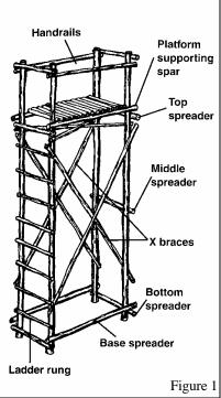
Mark 10' from the butt end of the 14' spars. This is where the **Top Spreader** (See Figure 1) will be placed. Lash a 3' spar to this location using square lashings. Ensure that you maintain the 2-1/2' separation between the 14' spars.
