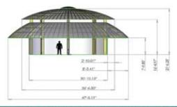
These are transparent dimensional renderings of a one and two level Chi'bagoda Perma Yurt based on a inner diameter of 30'.
