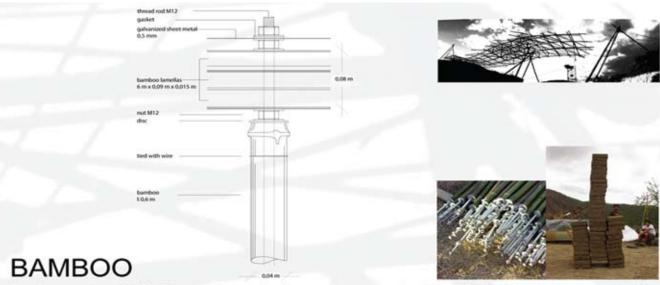
Bamboo was tested via 1:1 experiments in micro and macro scale; during the whole building process alternatives were tested to reach the wanted quality by exploiting the full potential of the material. The use of split Bamboo enabled us to create a free form surface structure, making full use of the materials ability to carry high tensile strength. "low tech" techniques helped to develop a feeling for the skills and limits of the material.
