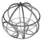
Coconut's concept aims to combine design and structure in a perfect balance. In order to achieve this result, coco features an innovative method of construction which employs only bamboo curved poles. The greater poles are curved while they are still growing, while the thinner ones are bended relaying only on the natural flexible power of bamboo. Like a basket, in coco every element plays a key role making harder the whole structure at every
