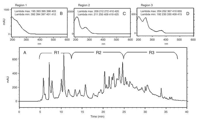
Figure 1. HPLC fingerprint of the *Syzygium cumini* aqueous leaf extract ( $\lambda$  = 280 nm; A) showing typical patterns of ellagitannins (B), gallotannins (C), and flavonoids (D) in the UV-visible absorption spectra.
