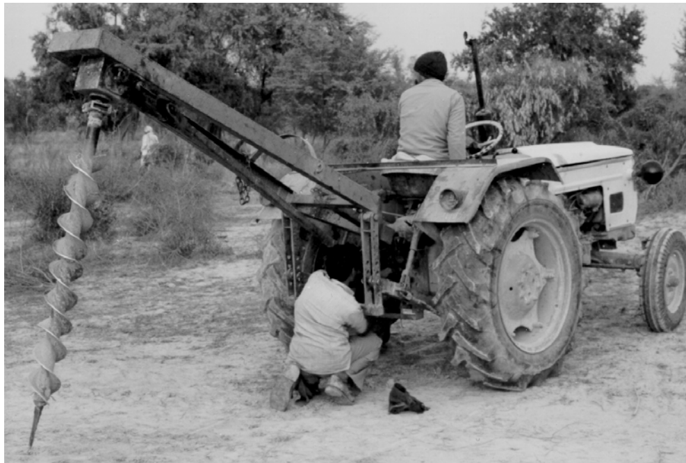
Figure 26. A tractor mounted auger for planting P. juliflora and other tree species in alkaline and other soils with a kankar pan.
