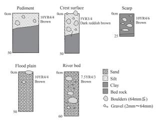
Fig. 3. Typical characteristics of soil cross-sections for each land unit.
