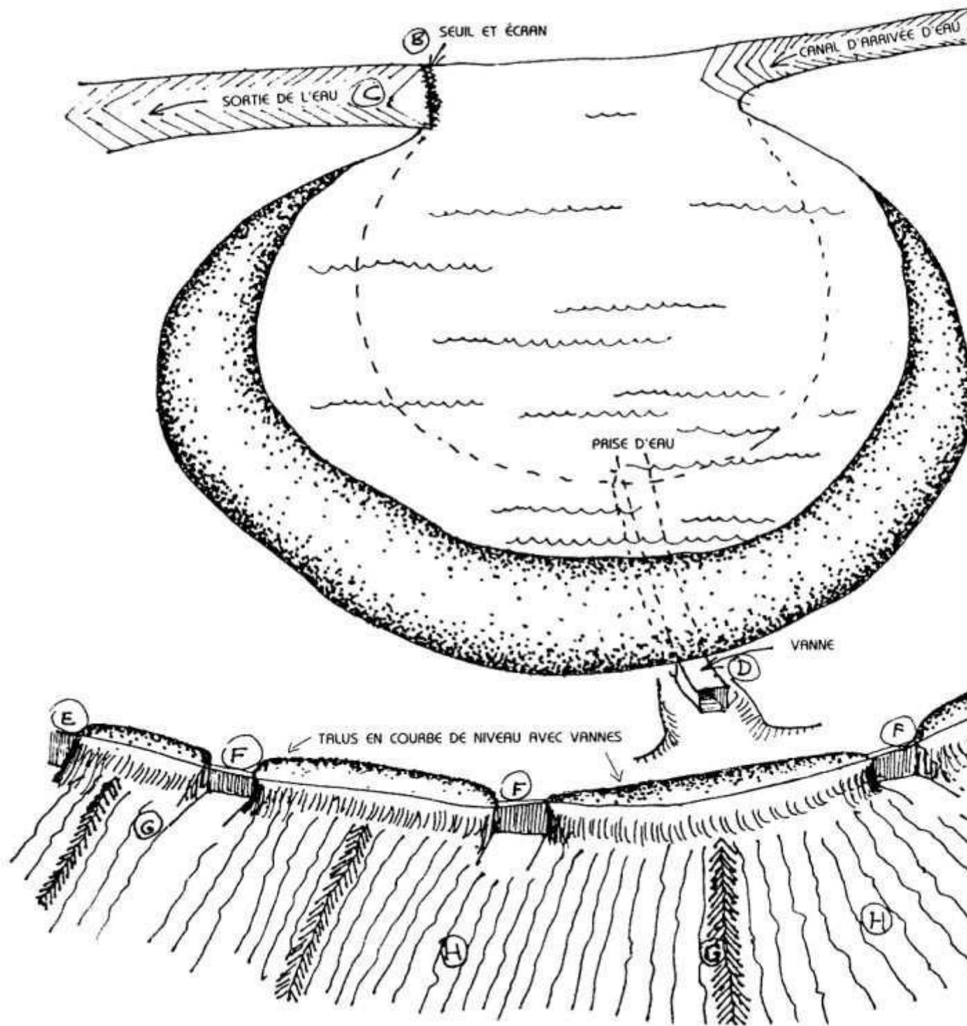
FIG. 7.14: LA RETENUE SUPÉRIEURE RECUEILLE L'EAU VENANT DE A PAR UN CANAL (DE DÉRIVATION) COUPANT LA PENTE. EN CAS D'INONDATION, L'EAU EN EXCÈS SE DÉVERSE EN B DANS LE CANAL DE SORTIE C OU PEUT ÊTRE RELÂCHÉE
