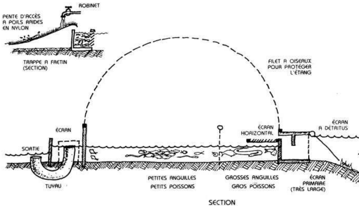
FIG. 7.23: SORTIE COMPLEXE POUR LA CAPTURE EN AMONT DE FRETIN ET DE CIVELLES, EN AVAL D'ADULTES (ANGUILLES ET AUTRES POISSONS). L'ÉTANG RETIENT LES ADULTES DESOENDANT VERS LA MER.
