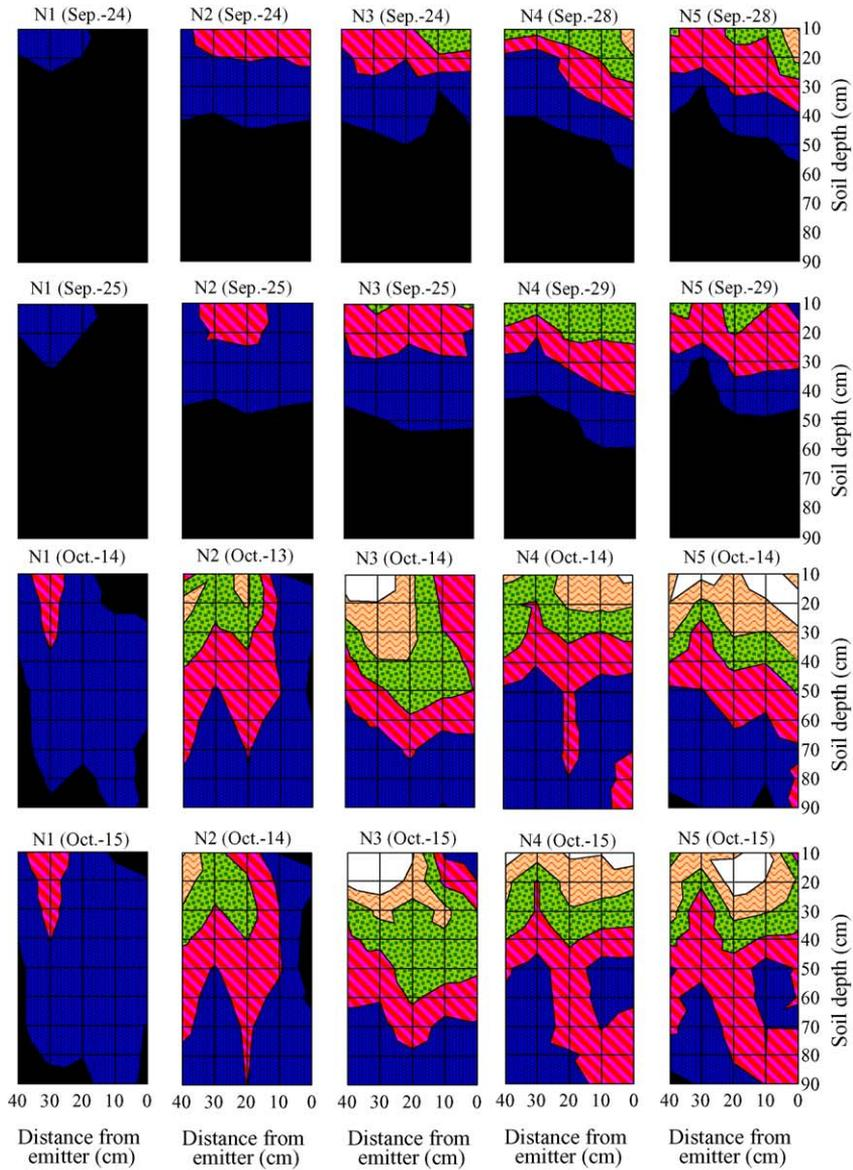
Fig. 6. Transect of spatial distribution of SWPs perpendicular to drip tape for different treatments before and after irrigation at leaf development and succulent root formation stages in 2002.
