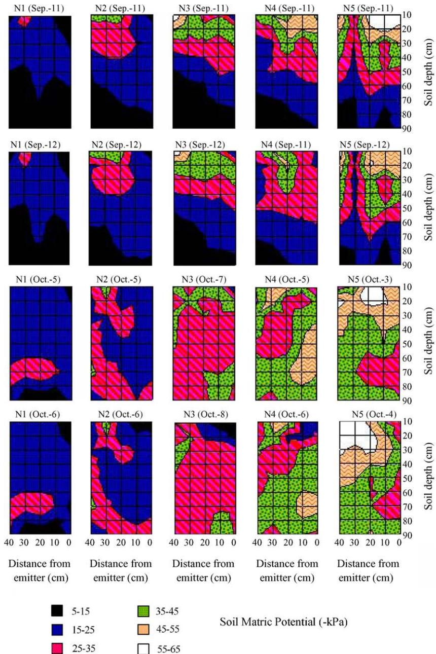
Fig. 5. Transect of spatial distribution of SWPs perpendicular to drip tape for different treatments before and after irrigation at leaf development and succulent root formation stages in 2001.
