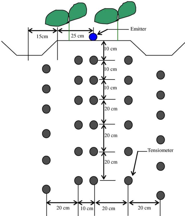
Fig. 1. Placement of tensiometers for each experimental treatment.
