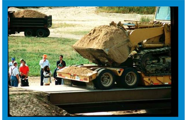
The composite bridge near Russell, Kansas, is load-tested shortly after its installation in 1996. Incorporating AOC resin technology, the bridge continues to pass load tests conducted periodically by the Kansas DoT.
