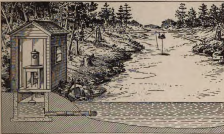
FIG. 9.—Equipment for river station, consisting of self-registering height gage, protected by small house with cable and car for convenience in velocity measurements.
