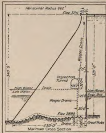
FIG. 47.—Typical section of masonry dam, Boise Project, Idaho.
