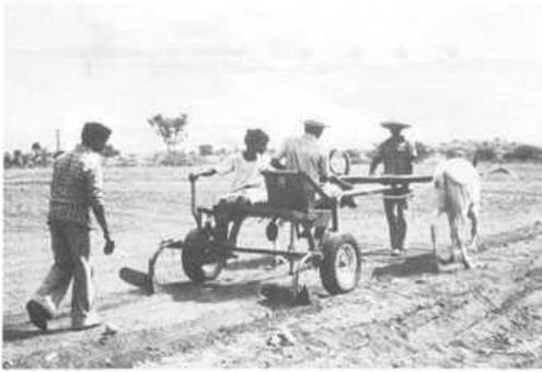
Plate 5.3 One of several tool carriers tested at ICRISAT for forming and cultivating beds (ICRISAT)
