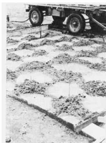
Plate 5.8 Experiments with artificial rainfall on 'tied-mounding', Burkina Faso (J. Collinet).
