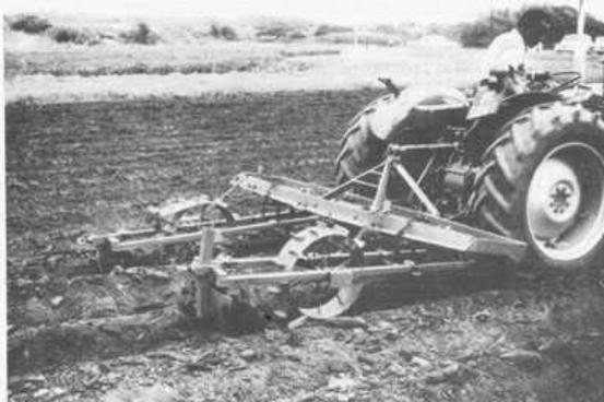
Plate 5.11 The ridger lifted by eccentric wheel (T.F. Shaxson)
