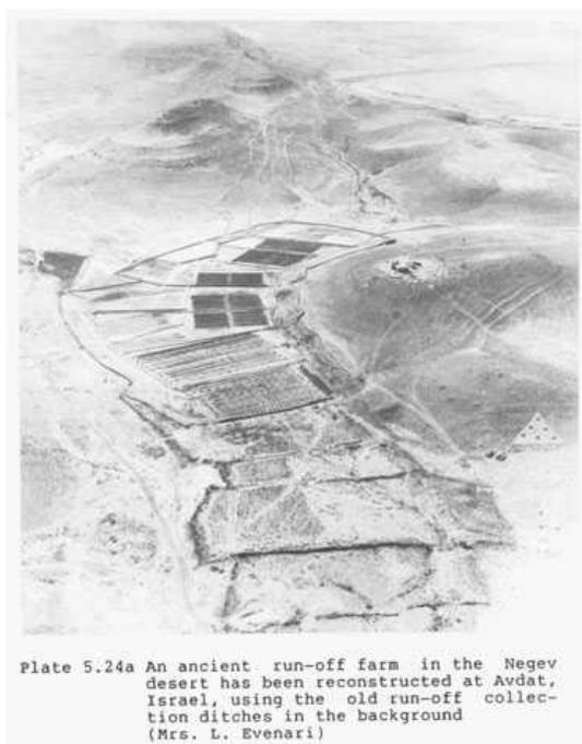
Plate 5.24a An ancient run-off farm in the Negev desert has been reconstructed at Avdat, Israel, using the old run-off collection ditches in the background (Mrs. L. Evenari)
