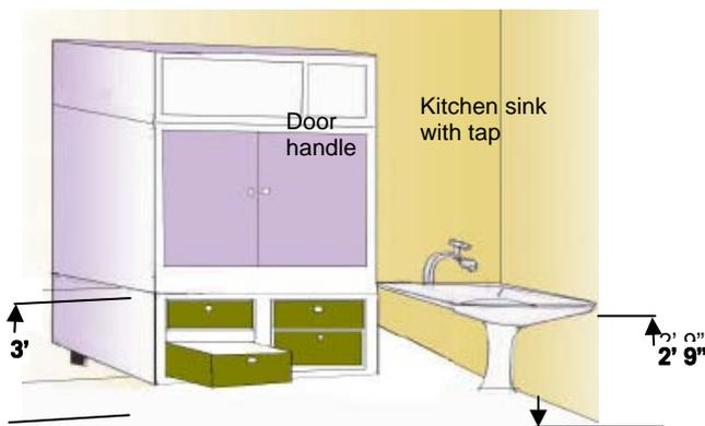
All pantry cupboards and sinks should be fixed at the given heights shown in Figure. 17.
