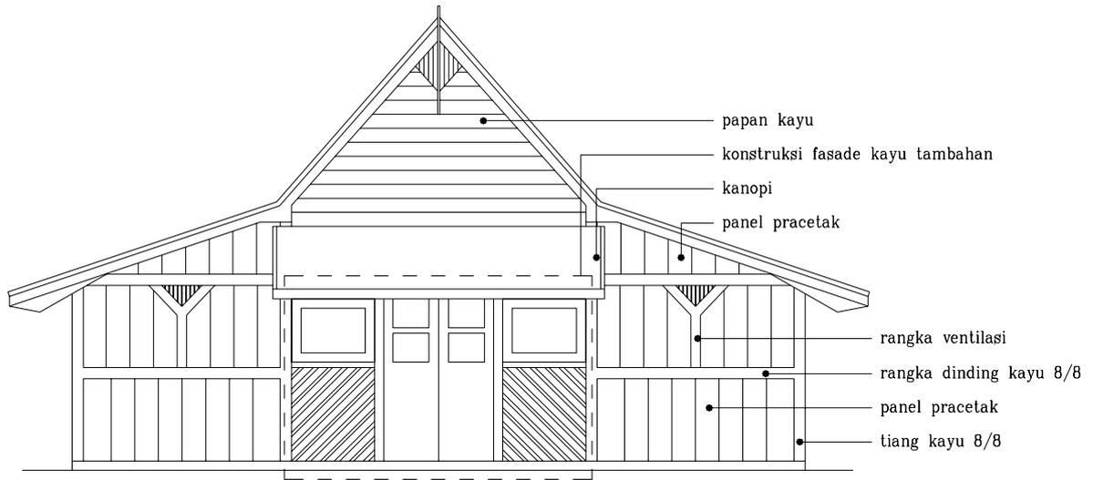
Front elevation of Gempol House. Precast concrete with bamboo reinforcement dominated the façade. Built in 1923, these 101 houses used to accommodate local colonial government employee in Bandung, West Java.
