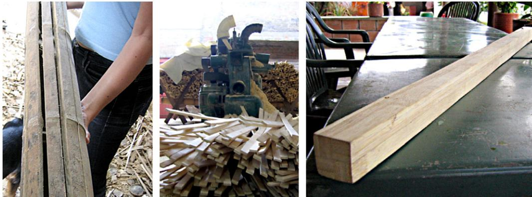
Fig. 1. From round bamboo to bamboo strips (‘latas’) to laminated bamboo beam/column. Source: Juan Ayala.
