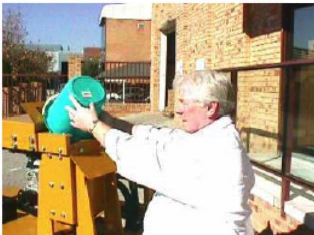
Filling the mold with treated soil
