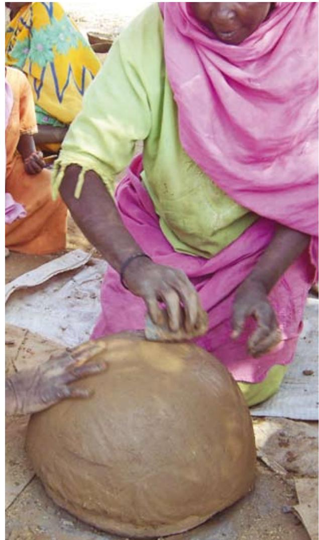
Pic 44. Using water and a stone the surface of the mixture is smoothed.
