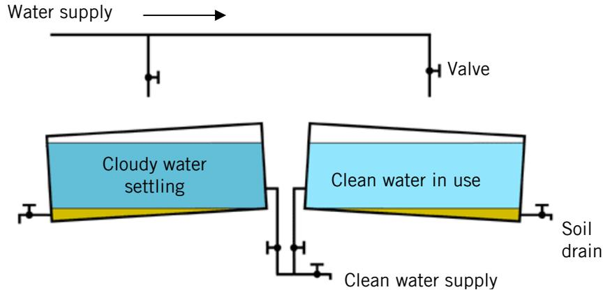
Figure 1: Double settling tanks arrangement. Clean water is taken from one tank while impurities are left to settle in the other.
