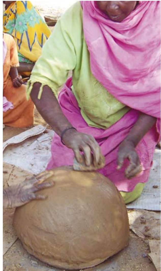
Pic 5. Using water and a stone the surface of the mixture is smoothed.
