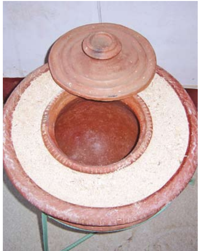
Pic 10. An assembled refrigerator using wood chippings for insulation.
