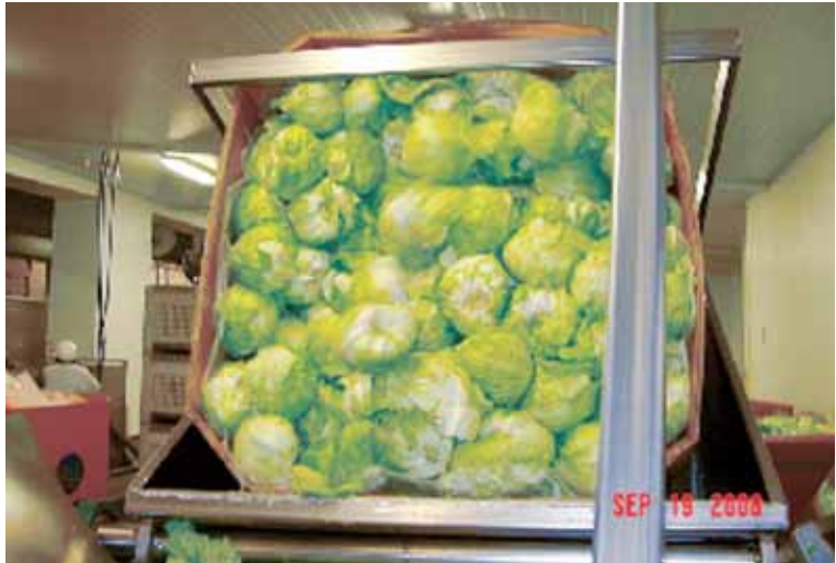
Plate 7.2 Product bin dumper (Image published with permission of Boskovich Farms, Inc., California, USA. www.boskovichfarms.com )
