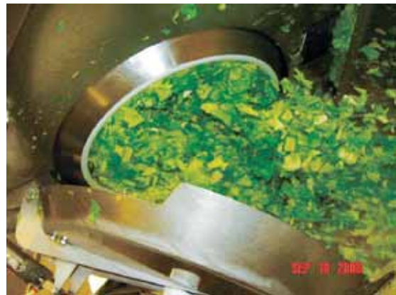
Plate 7.3 Product cutting and slicing machine (Images published with permission of Boskovich Farms, Inc., California, USA. www.boskovichfarms.com )
