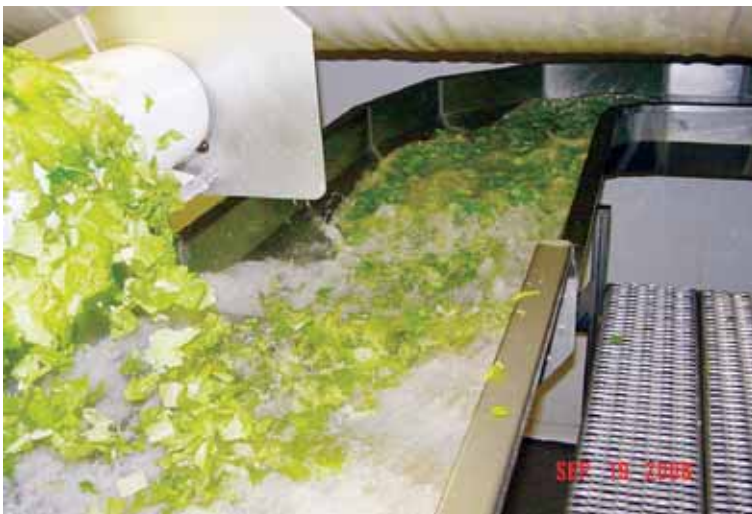
Plate 7.4 Continuous product washing flume (Image published with permission of Boskovich Farms, Inc., California, USA. www.boskovichfarms.com )
