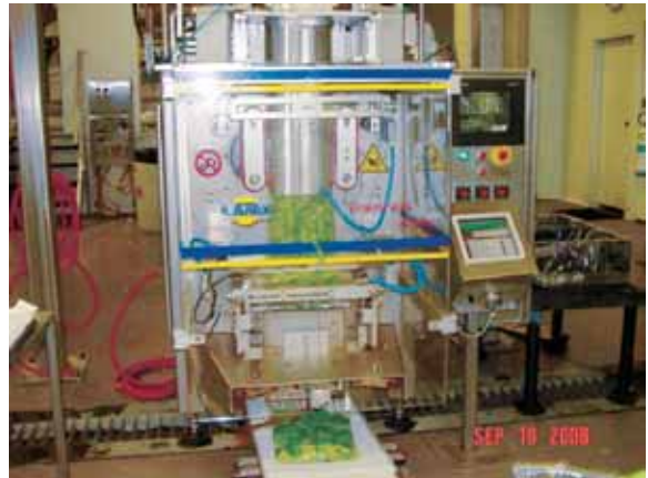
Plate 7.6 Auto scale with form-fill-seal packaging unit
