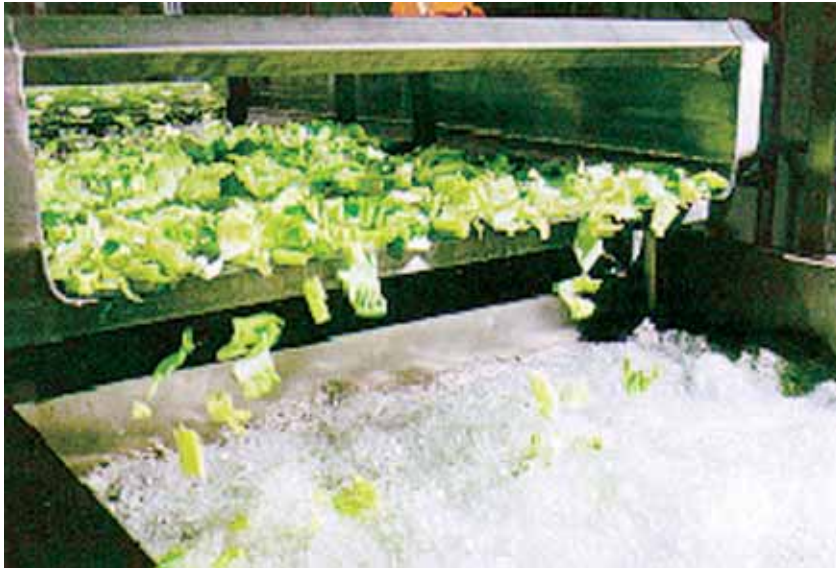
Plate 6.3 Continuous washing of pre-cut lettuce
